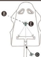
**6. Insert the backrest mount into the hole in the butterfly mechanism and secure it by turning the handle.**
